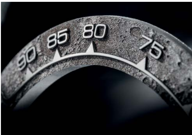
Moon-like surface texturing on a watch bezel. Source: LASEA.
