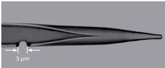
Glass needle microdrilling. Source: Workshop of Photonics.
