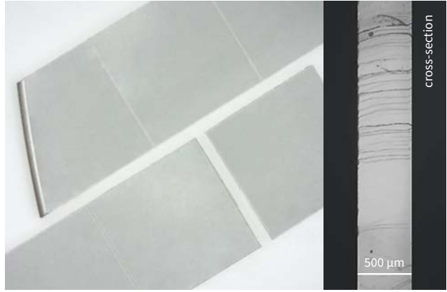
Single-pass (300 mm/s) dicing of 500 µm thick 4H-SiC wafer.
