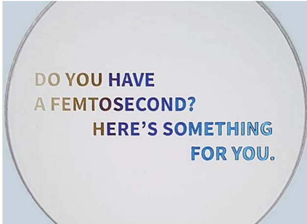
Form induced birefringence-retardance variation results in different colors in parallel polarized light. Source: Workshop of Photonics.
