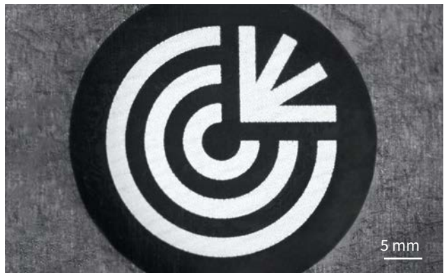
High-contrast black-and-white marking on stainless steel clips using the BiBurst option.
