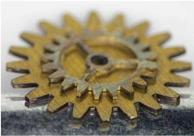
Cut and welded parts from brass using a single laser system.
