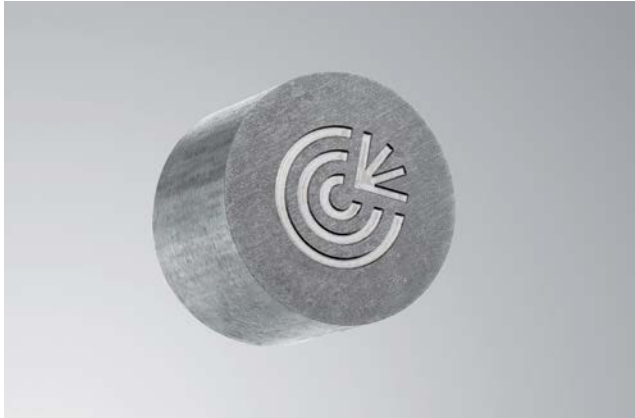
Selective ablation of tungsten carbide.
