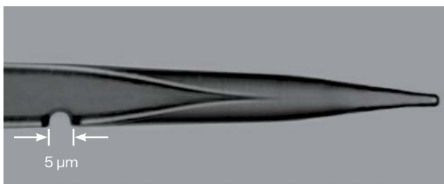
Glass needle micro-drilling.
