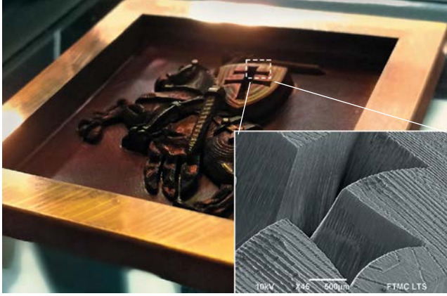
3D-milled sample in copper. Zoom-in SEM image.
