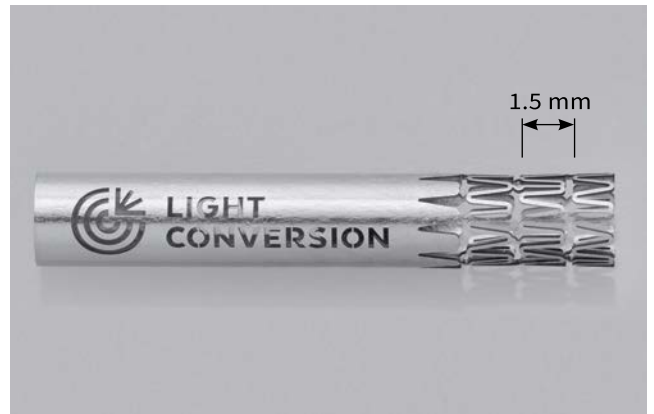
Example of a stent cut from stainless steel.
