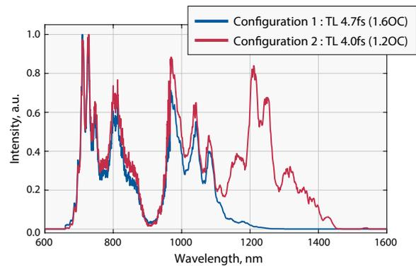
Spectra of pulses produced by OPCA frontends, two configurations are available
