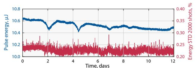
Energy and energy stability of the passively CEP stabilized pulses generated in an OPCA frontend measured over 12 days
