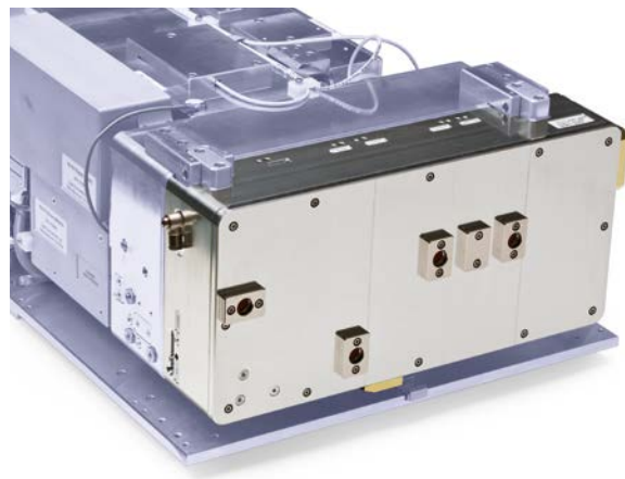
Fixed wavelength I-OPA-FW module attached to PHAROS
