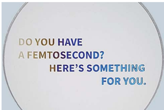
Form induced birefringence-retardance variation results in different colors in parallel polarized light.
